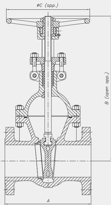
Carbon steel and alloy steel construction
