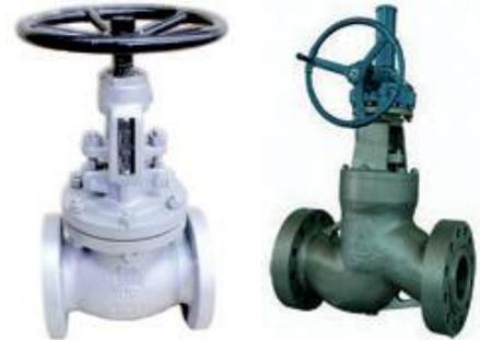
All globe valves utilize the “port closure” concept of valves. By this it meant that fluid passes through a specific opening (rather than a general passageway, as in the case of gate valves), and the fluid is controlled by means of a stem-mounted disc or inserted plug in that area.
